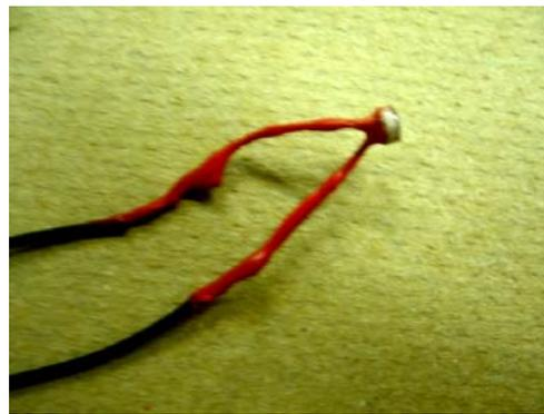
5) Solder the resistor to the other end of the hook-up wire connected to the longer lead of the NXT (the one you marked with a red blob in step 1). (If you forgot to mark the wire and now you can't tell which lead is which, ask your teacher for help).
