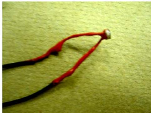
5) Solder the resistor to the other end of the hook-up wire connected to the longer lead of the NXT (the one you marked with a red blob in step 1). (If you forgot to mark the wire and now you can't tell which lead is which, ask your teacher for help).
