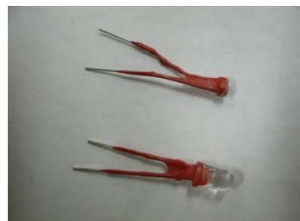
2) Solder each of the LED legs to a piece of hook-up wire. CHECK WHICH LED LEG IS LONGEST, AND LABEL THE HOOKUP WIRE CONNECTED TO IT (for example, you could use a blob of liquid tape, as shown). Later we will have to be careful to connect the LED across the NXT the right way round-it only works one way and not the other.
