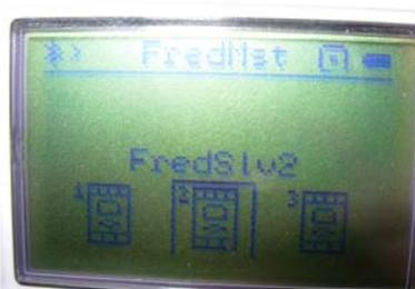
Inside the master's connections list: We see that FredMst is connected to three slaves. We can also see that FredSlv2 is assigned to address no. 2.
