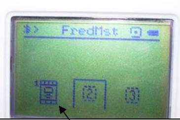
FredMst is now connected to a slave NXT at address no. 1. Addresses 2 and 3 are still empty.
