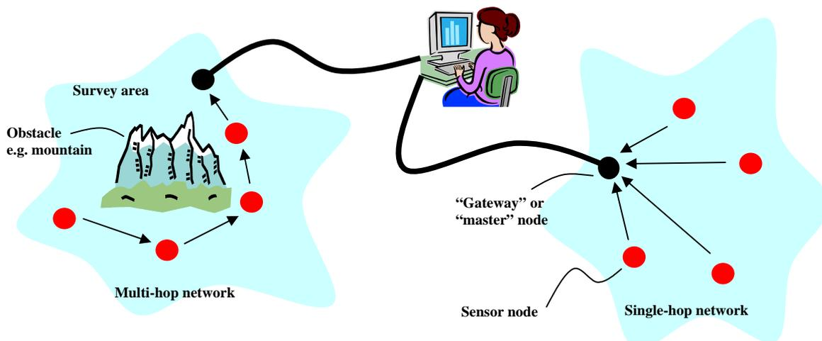
Figure 1. In a “single hop” network (right), each sensor node transmits its data directly back to a gateway node, from which it can be delivered to the scientist’s computer for analysis. If the data has to be transmitted over very large distances, or around an obstacle, then it may be necessary to use a “multi hop” network (left) in which data is relayed from one node to the next along a chain of communicating way-stations.
