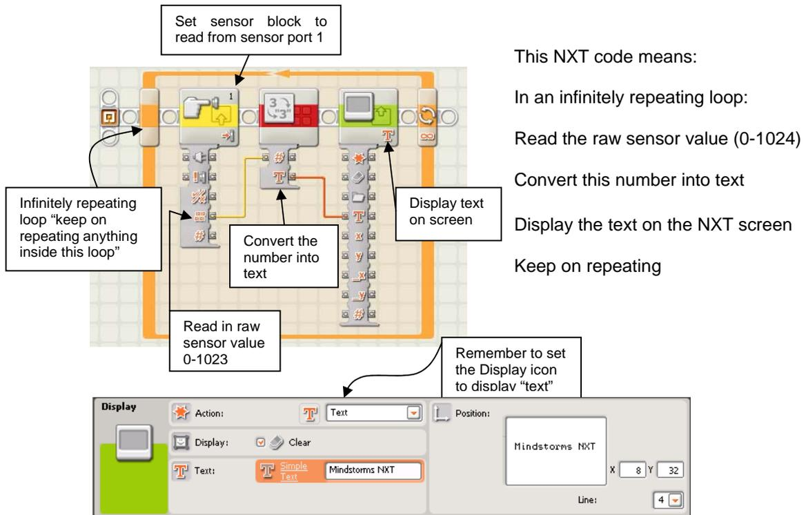
Caution: **do not** use the ready made “temperature sensor” icon that is built in to the NXT programming system. This is designed for use with the LEGO temperature sensor which has different calibration characteristics from the sensor you are building. Therefore the NXT temperature sensor icon may give false temperature readings if you try to use it with your own thermistor.
