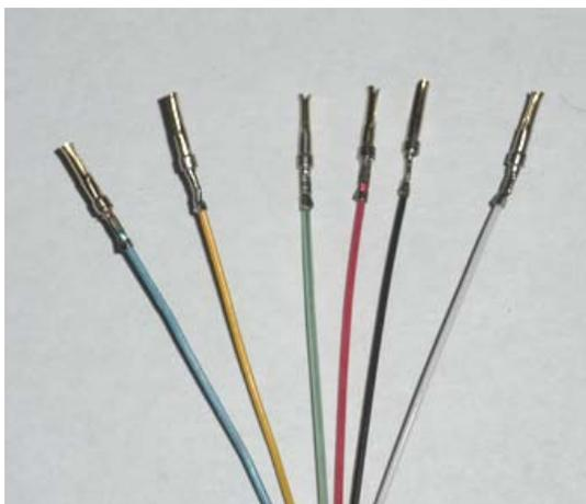
Load a male D-sub connector pin into the 20-24 AWG slot of the D-sub crimper. (If this slot is not available, stick with the 24-28 AWG slot.) Be sure to insert the pin so that the opening is facing down. Squeeze the crimper slightly to secure the pin in place.
