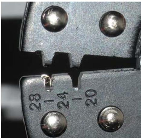
Take one of the conductors from the RJ12 telephone cable and carefully slide it into the pin so that only a very small amount of insulation is inside the pin. Then squeeze the crimper tightly to secure the pin to the cable.
