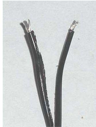
Use the wire stripper to strip about 2 mm of insulation from each of the conductors at the other end of the 4-5 meter RJ12 telephone cable.
