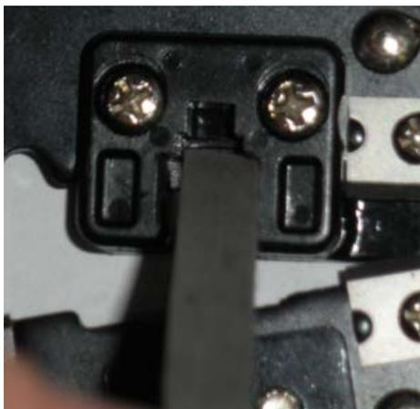
Be careful! If you remove too much material, the crimper will not work correctly and will actually damage your plug. The best way to go about this is to remove some material and then try to put the plug in. If it won't go, then file some more and try again.
