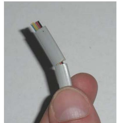
Use the needle nose pliers to pull out the white and black conductors from the insulation.
