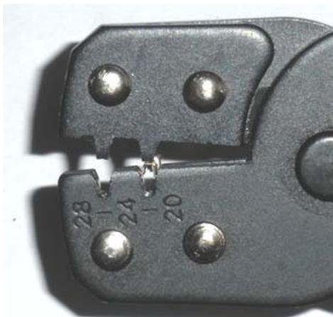
Take one of the conductors from a 1280 mm connecting lead and carefully slide it into the pin so that only a very small amount of insulation is inside the pin. Then squeeze the crimper tightly to secure the pin to the cable. Open the crimper and carefully remove the pin. As before, the back part of the pin should be latched onto the insulation and the thinner section towards the middle should be latched onto the bare wire.
