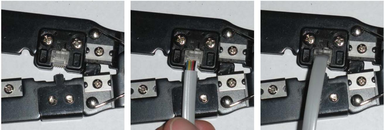
Make sure the cable is pushed all the way into the plug and then squeeze the crimper down on the plug. If you look at the other end of the crimper while you do this, you will see the crimper's teeth push in the blades of the plug into the wires inside.
