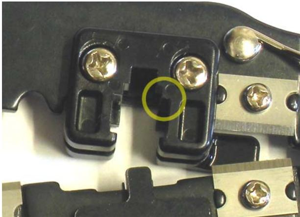
There is a space in the center for the latch from a regular RJ12 telephone plug, but the NXT latch will hit against the right side and won't fit into the crimper. The only way to solve this problem is to file away the extra material on the right so that the NXT plug will fit.
