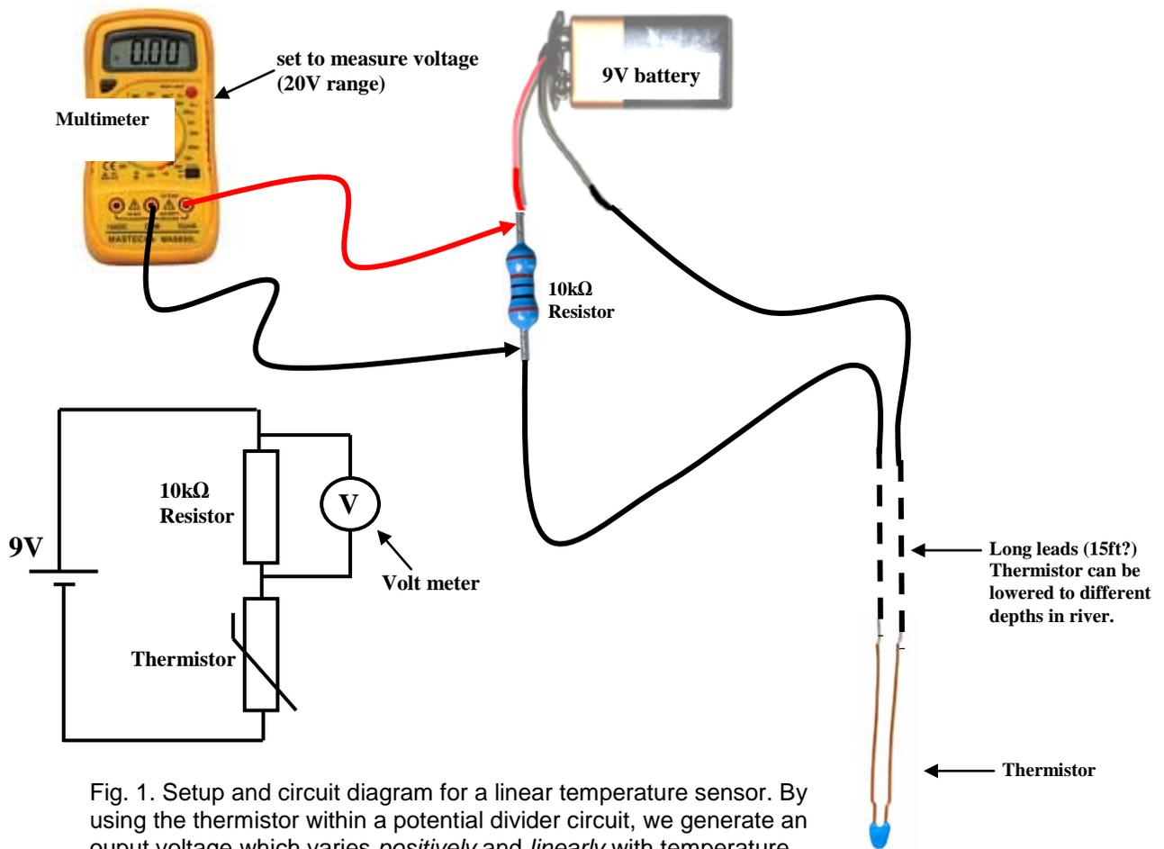
Fig. 1. Setup and circuit diagram for a linear temperature sensor. By using the thermistor within a potential divider circuit, we generate an output voltage which varies *positively* and *linearly* with temperature.
