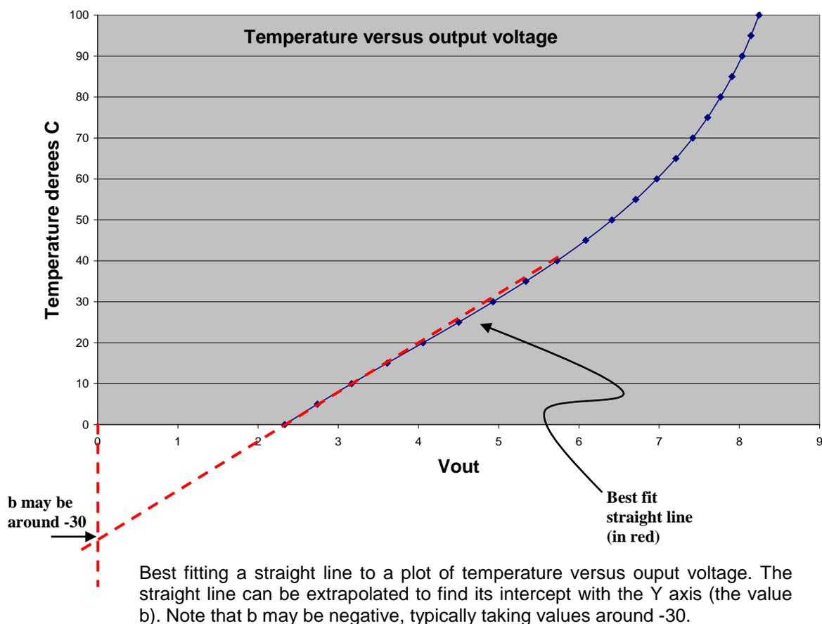
Calculating the values of  $m$  and  $b$  is really the process of **calibration**. You have now found a simple formula which relates any sensor output,  $V_{\text{out}}$ , to Temperature (the quantity you want to measure). Now you can use your sensor system and your equation 1 to measure new unknown temperatures in the environment.
