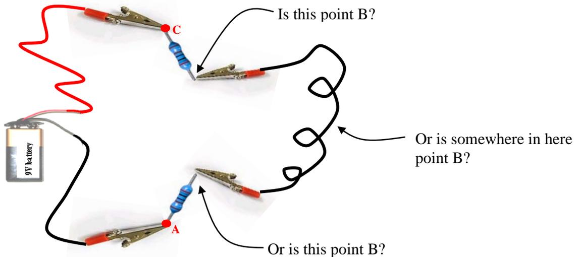
The answer is that it doesn't matter. All of these points are electrically equivalent. They are all point B and will all measure the same voltage. We assume that the wires which connect components are perfect conductors with negligible resistance. Therefore it is only the components themselves that are important. The wires that connect them can be
