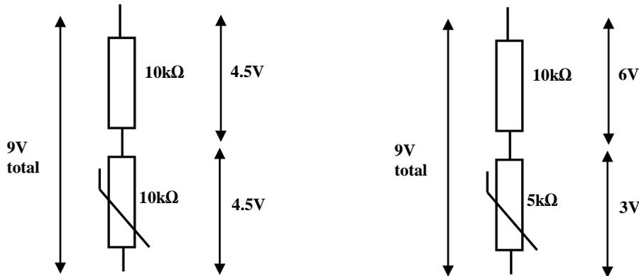
Fig. 2. A voltage divider divides the total voltage up between the two resistors in proportion to their resistances.
